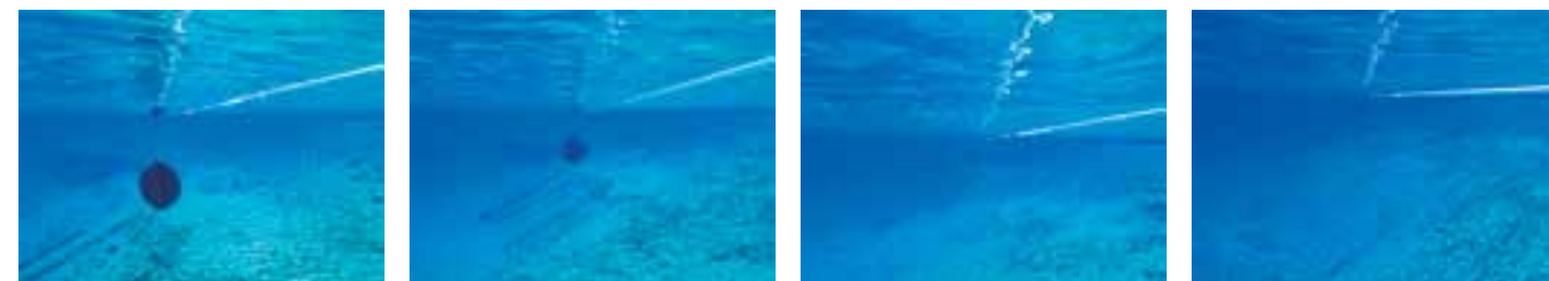
Researchers gauge clarity by examining visibility of a black disk across a horizontal distance, pictured here at 7, 18, 35 and 50 meters.
