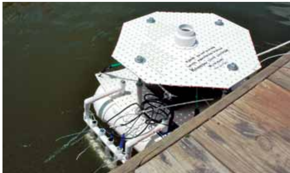
The standard Basic Observation Buoy build plan calls for pegboard and PVC.
