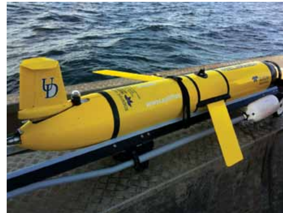
OTIS - a Slocum glider - picks up signals from acoustic transmitters implanted in sturgeon and measures water quality parameters.
