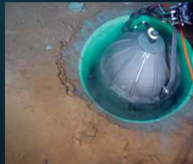
Clockwise from top: The remotely operated vehicle ROPOS being recovered by the R/V Thomas G. Thompson with a short period seismometer package; One of eight seismometers installed at an ocean spreading-center volcano 150 miles off Vancouver Island; A Guralp broadband seismometer installed in a MBARI invented housing placed into a hole in sediments on the seafloor.
