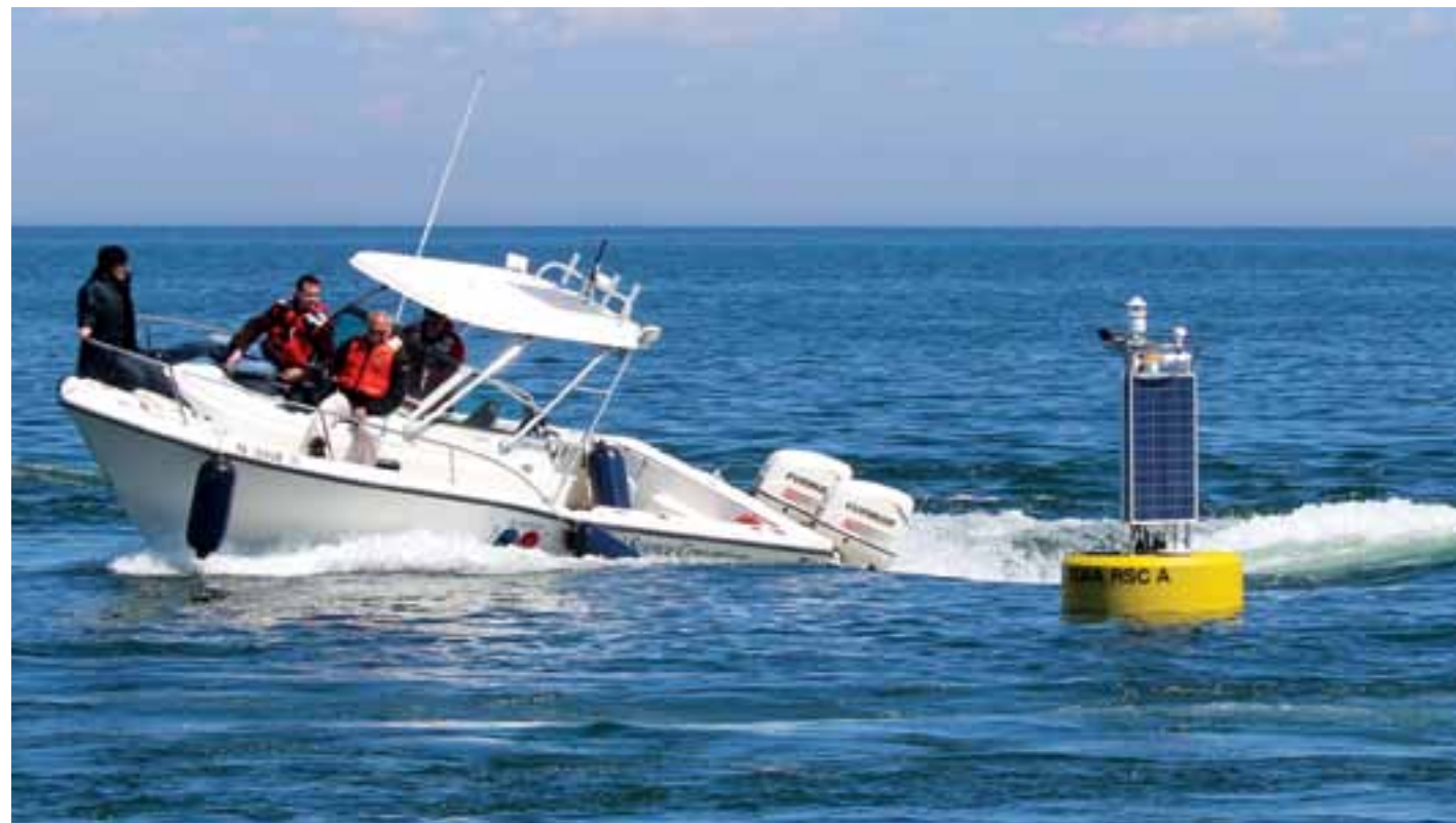
Stirring up some wake to test the buoy's wave measurement capabilities.
