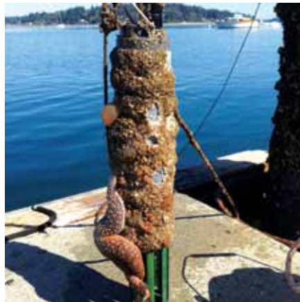
Intense biofouling on multi-parameter sensor.
