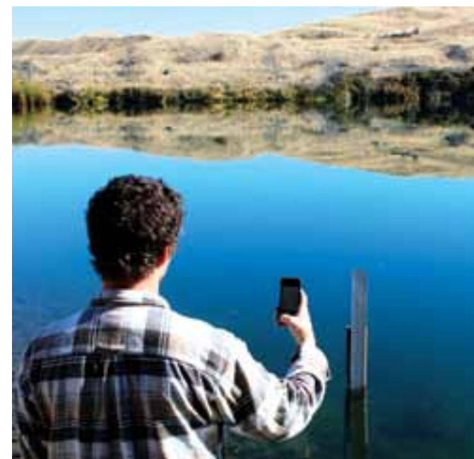
MobileTracker calculates discharge from staff gauge photos.
