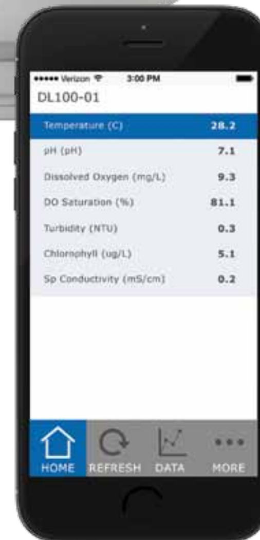
The NexSens DL100 (actual size shown) connects wirelessly to a smartphone for quick setup, troubleshooting and data readings.
