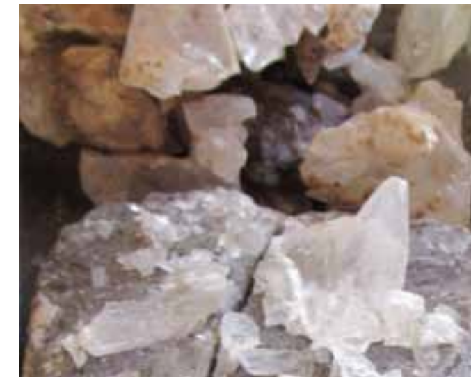
Gypsum crystals precipitated on a natural fracture in the Tucucaro ignimbrite at around 100 meters depth.
