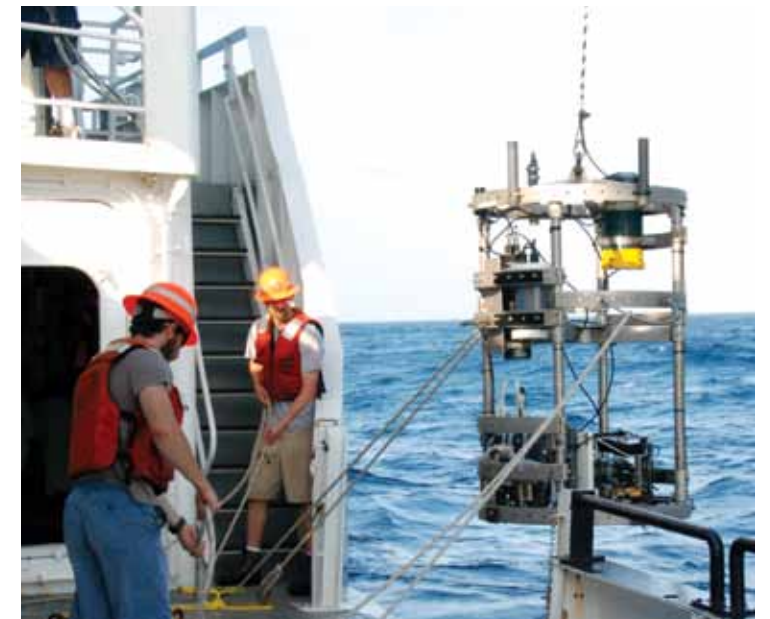
Oceanographers deploy a chi-pod sensor and other instruments to measure conductivity, temperature and depth.
