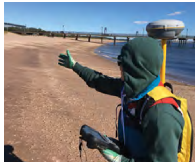
Clara Holmes uses an RTK GPS for shoreline monitoring to get accurate geolocations of the wrack line on the beach after storms.
