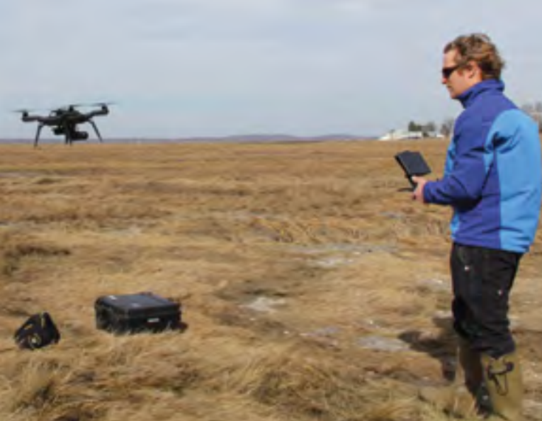
Moore launching a vegetation mapping UAV (3DR Solo) outfitted with a pair of MAPIR Survey3 high-resolution cameras to capture RGB (visible light) and NDVI imagery.
