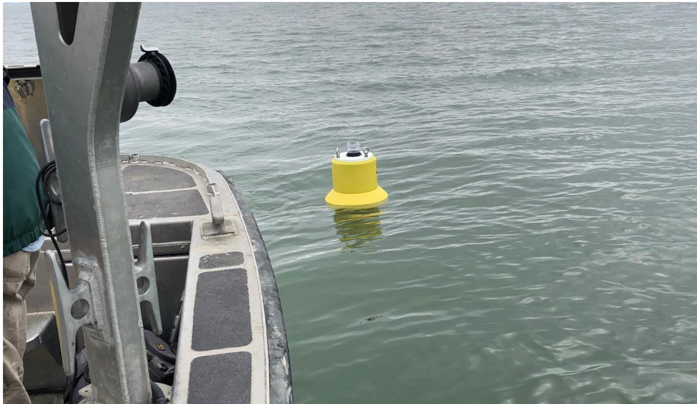
A NexSens CB-50 monitoring buoy collects water quality data in the shoals of San Francisco Bay.
