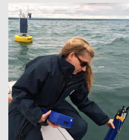
Jeanette Schnars, executive director of the Regional Science Consortium, collects water quality data near one of the center's buoys that help track temperature, pH and turbidity.
