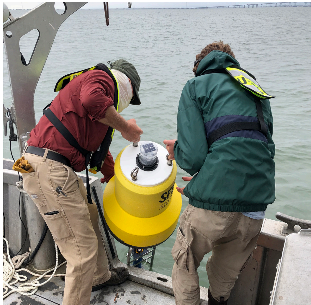
USGS California Water Science Center personnel (Sacramento) deploy a NexSens CB-50 buoy with YSI EXO2 multi-parameter water quality sonde.
