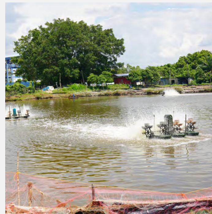
(Left) Aeration to provide sufficient oxygen to cultured animals. IoT can monitor low oxygen levels and give warning or switch on the aerators to overcome the problem.
