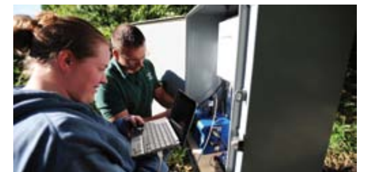
Claire Weldon, Cleveland Metroparks aquatic research coordinator, runs diagnostics on an Isco flow meter at a wetlands monitoring station.
