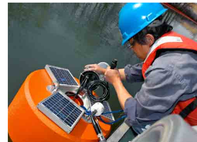
NexSens Chief Technical Officer Doug Nguyen installs a submersible data logger into an MB-300 data buoy.
