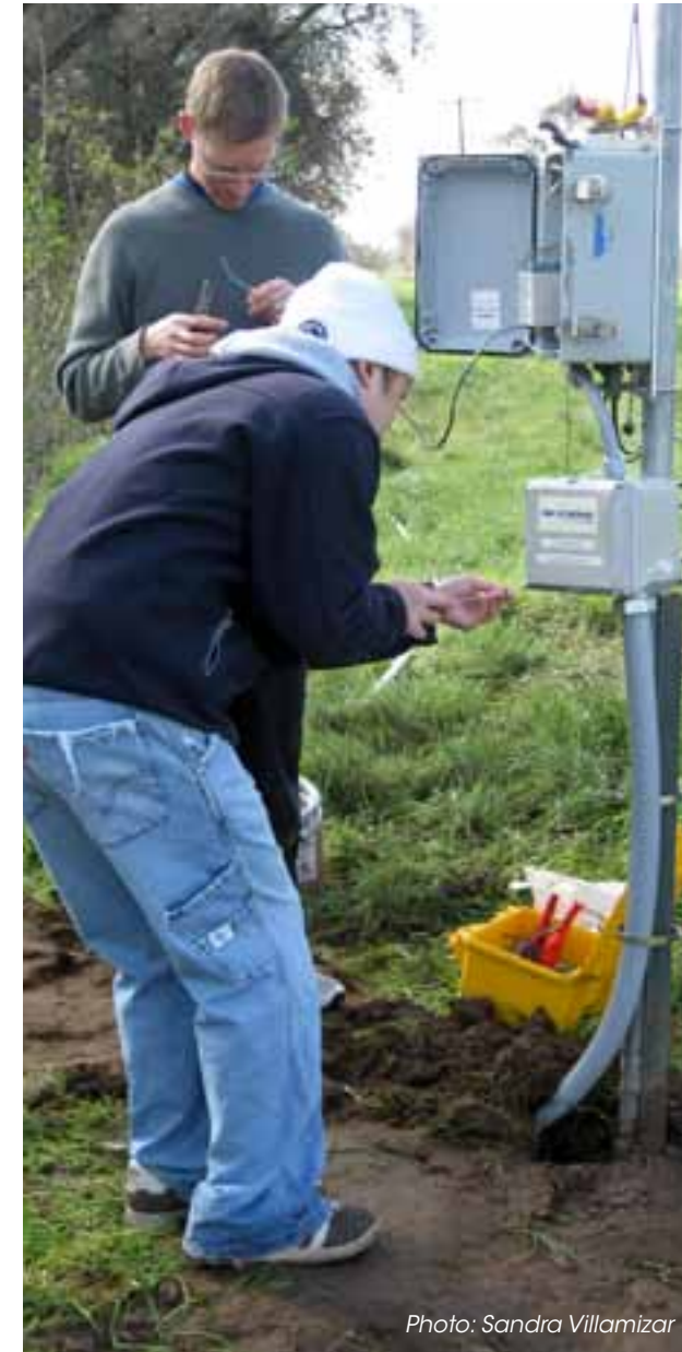
Researchers install a cellular telemetry system to transmit data in real-time.
