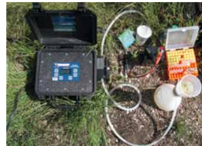
The researchers now use a Pegasus Athena peristaltic pump to make sampling easier and more efficient.
