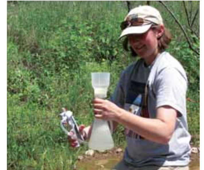
Caren Glodberg pumps a water sample through an eDNA filter.
