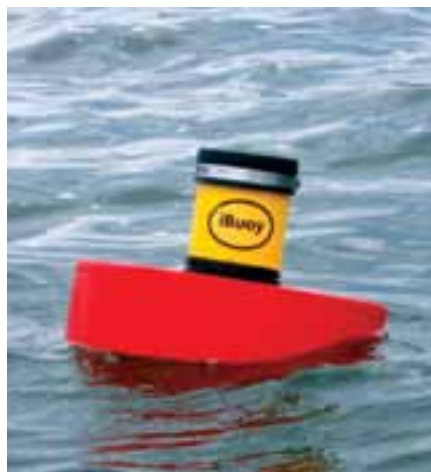
The IBuoy measured wave height in Chesapeake Bay.
