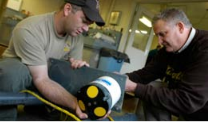
Fisheries Biologist Travis Hartman works with a NexSens field engineer to mount an acoustic Doppler current meter.
