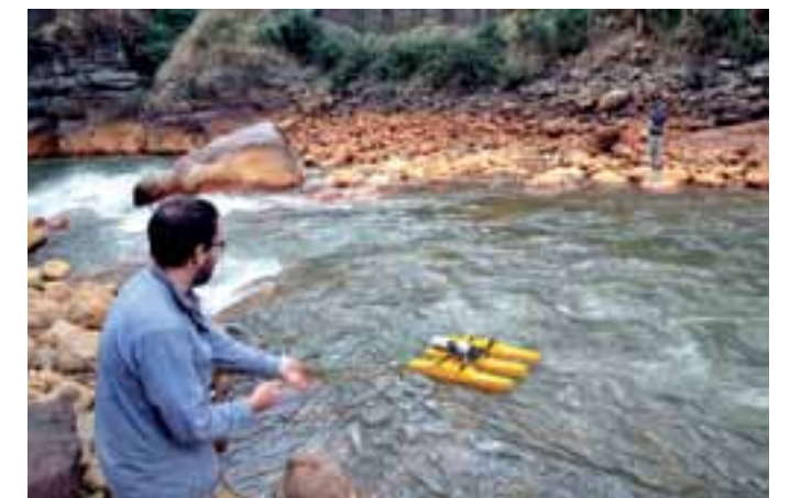
Researchers towed the RiverSurveyor across the Rio Santa, gathering discharge data to calibrate a network of stream gauges.
