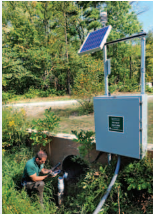
Michael Durkalec with Cleveland Metroparks services a water quality sonde at a stormwater monitoring site.
