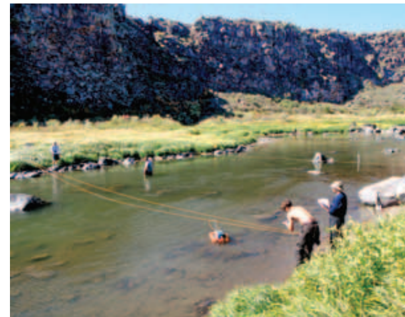
The crew's pulley system towed the ADCP back and forth across the channel for quick measurements that would have taken hours with a traditional meter. Photo: Paul Bauer
