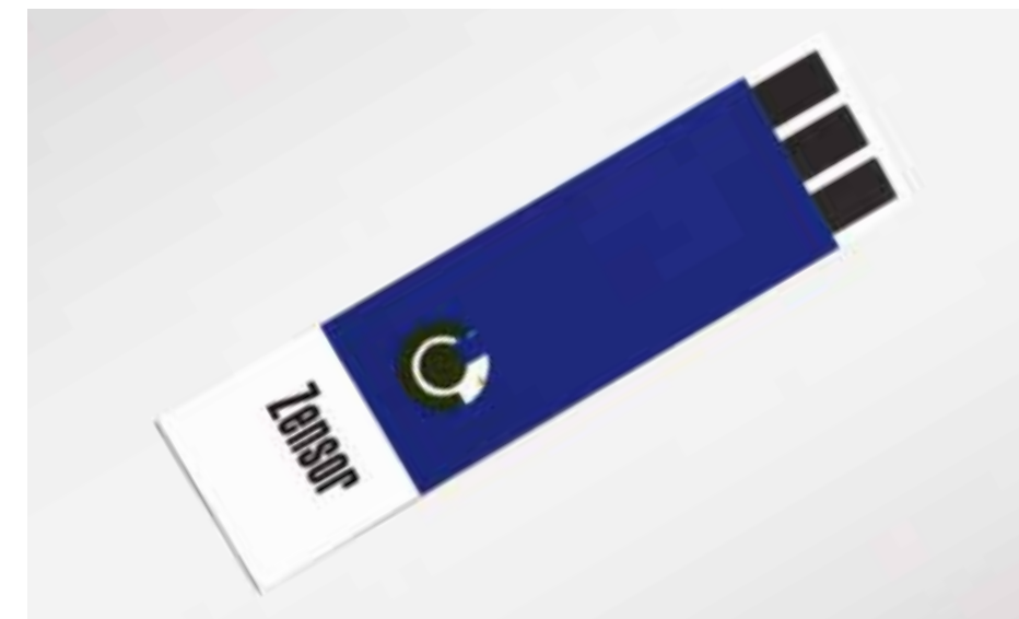
Screen printed electrode used in detecting green leaf volatiles.
