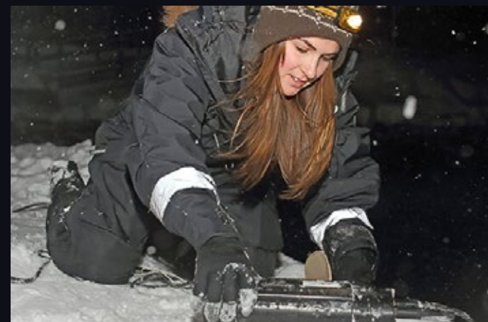
Graduate student Heather Cronin deploying a bathyphotometer to measure bioluminescence.
