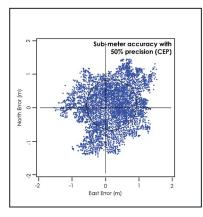
plot points within a meter radius of the true point. However, those points may only fall within that meter radius, 50–60% of the time. The accuracy for those receivers is sub-meter, but the precision is only 50–60%.
