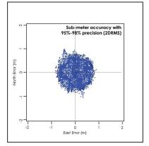
For the Geode in ideal conditions, 95–98% of the points on a scatter plot will fall within a sub-meter radius of the true point.
