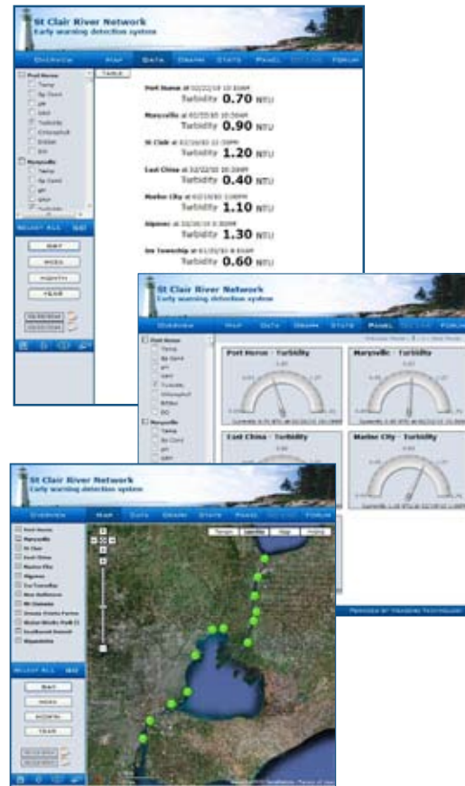
NexSens WQData software displaying area maps, historical data, and current readings for a project site.
