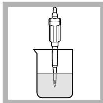
**4.** Put the probe in the first pH buffer solution. Make sure that the sensor and reference junction are fully in the solution. Do not put the probe on the sides or the bottom of the beaker.
