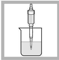
2. Put the probe in the sample with the sensor and reference junction fully in the sample.
