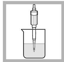
4. Put the probe in the pH buffer solution with the sensor and reference junction fully in the solution. Do not put the probe on the bottom or sides of the beaker.
