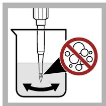
5. Shake the probe from side to side to refresh the reference junction and remove air bubbles.
