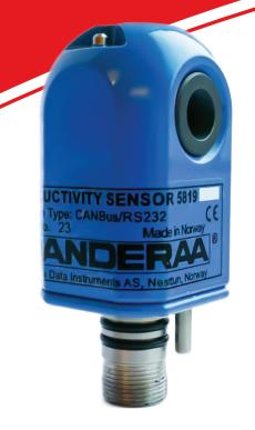
Conductivity Sensor 5819/5819R is a compact fully integrated sensor for measuring the electrical conductivity of seawater. Designed to be used with SeaGuard or SmartGuard data logger using AiCaP CANbus or as stand-alone sensor using RS-232/RS-422
