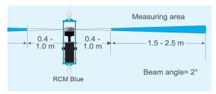
The solid state sensor is well suited for monitoring low current speeds due to no moving parts. Because the sensor starts measuring in an area 0.4 to 1.0 meter from the instrument, the effect of marine fouling and local turbulence is minimized.
