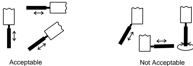
Figure 1 – Correct and Incorrect Angles of Measurement
