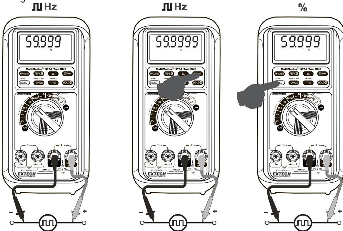
Note: Unlike the Line Level Frequency measuring function as previously stated, this Logic Level Frequency function is set only at the highest input sensitivity for measuring digital type electronic signals.
