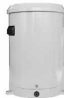
Each unit consists of a collector funnel with leaf filter, an integrated syphon control mechanism, an outer enclosure with quick release fasteners, and base which houses the tipping bucket mechanism. The rain gauge also includes dual output reed switches with varistor protection that senses the pulse from each tip and logs it in an internal or external data logger. The dual reed switch can also transmit the tipping bucket pulse from the rain gauge to a telemetry system.
