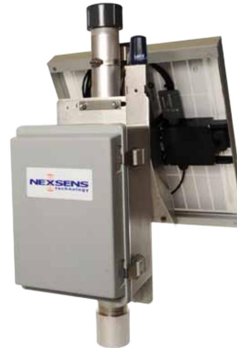
The iSIC-MAST system includes the data logger and solar panel pre-mounted to a 2" diameter pole to create a truly plug-and-play data collection and sensor interface platform. The system integrates a NexSens iSIC data logger and 20-watt solar power kit - all in a compact, pre-configured package. Simply thread the system to any 2" NPT male pipe thread, connect the solar panel & battery, wire the sensors, and setup a project using iChart software - it's that simple!
