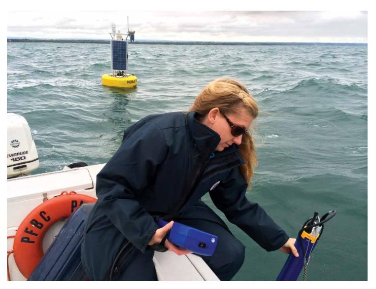
ferent sensing instruments. The sonde or sensor can be lowered into the water column to a depth that matches the in-place sensors. While it is at that depth, a water quality measurement can be taken. The data from this portable system can then be compared to the in-place monitoring system and checked for discrepancies.
