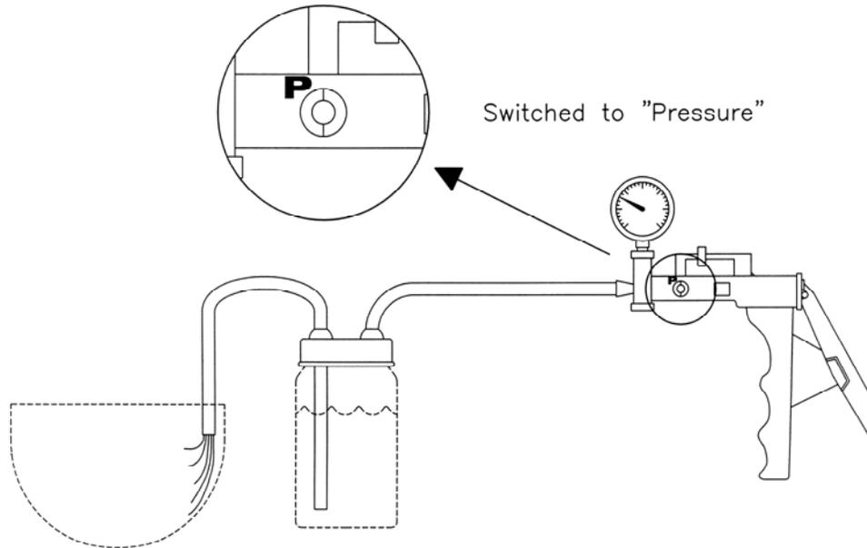
**Figure 2 – Liquid Transfer Procedure**
