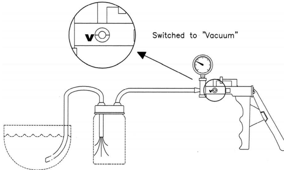
Figure 1 - Siphoning Procedure
