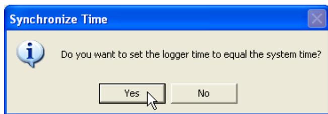
**Sync Time:** This button causes the data logger’s internal clock to be set to the system time of the computer it is connected to. The user is warned first and must confirm the action before the time is set.
