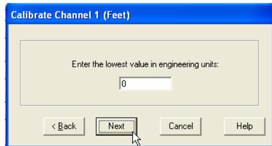
Place the sensor in the condition that will cause it to output the level corresponding to the low EU entered in the previous menu. Wait for the data reading to stabilize. Click Next to complete the calibration.
