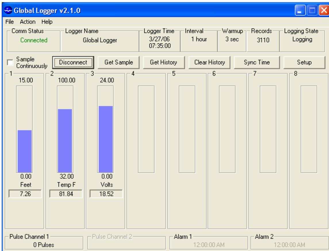
The functions and information in this screen are discussed in the following sections. The screen image above shows water level and temperature although any type of sensor can be connected to the logger. Battery voltage is always monitored on channel 3.
