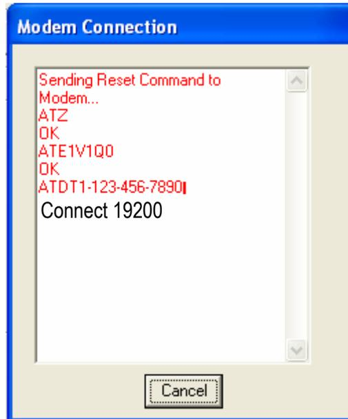
Once a connection is established, “Connect” will appear for a few seconds along with the baud rate of the connection. After connecting, the normal Global Logger screen will appear and operate exactly as if a direct connection was made. All options and features work the same but at a reduced communication speed.
