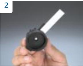
2. Verify that the test strip pad is positioned over the hole.
