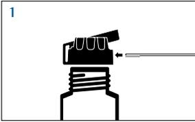
1. Lift the flap on the black cap and slide a test strip into the groove so that the reactive pad faces the small opening and completely covers it; secure by pressing the flap back into place.
