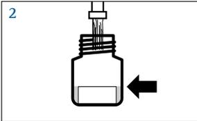
2. Fill the reaction vessel with sample water to the top edge of the label (50 mL).
