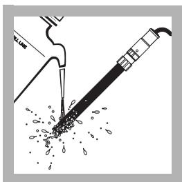
6. Rinse the electrode in deionized water and blot dry.
