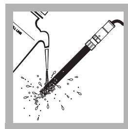
12. Rinse the electrode with deionized water followed by a small amount of sample and blot dry.
