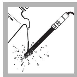
8. When a stable pH is determined, the display will show **Standard 2?**. Remove the electrode from the cup. Rinse and blot dry.
