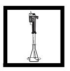
**3.** Titrate with sodium hydroxide from colorless to a light pink color that persists for 30 seconds. Record the number of digits required.
