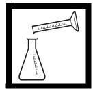
**4.** Use a graduated cylinder or pipet to measure the sample volume from *Table 1* or *Table 2*. Transfer the sample into a clean 250-mL Erlenmeyer flask. Dilute to about the 100-mL mark with deionized water, if necessary.
