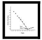
**11.** Using linear graph paper, plot the recorded readings from the Amperometric Titrator on the vertical axis and the corresponding Digital Titrator digits on the on the horizontal axis. Draw the two best intersecting lines through the points see *Figure 1*. Determine the number of digits at the intersection of the lines; this is the end point.
