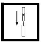
**3.** Using the 3-mL (3-cc) syringe, collect a 2.0-mL water sample. Add to the vial provided.
