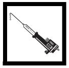
**8.** Flush the delivery tube by turning the delivery knob to eject a few drops of titrant. Reset the counter to zero and wipe the tip.
