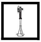
tube tip into the solution and swirl the flask while titrating with EDTA from red to pure blue. Record the number of digits required.
