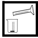
**3.** With minimum agitation, measure 200 mL of sample with a clean graduated cylinder. Transfer the sample to a clean 250-mL beaker containing the 50-mm stirring bar supplied with the system.
