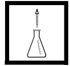
**9.** After completing the calcium titration, add 1 mL of 5.25 N Sulfuric Acid Standard Solution. Add additional acid dropwise and swirl the solution until the color changes from pure blue to purple, then to blue and finally to red. Swirl the flask to ensure that all precipitated magnesium hydroxide has redissolved.
