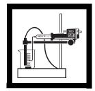
**2.** Install the Standard Iodine Titrant Cartridge, 0.028 N. Flush the Digital Titrator delivery tube by turning the delivery knob to eject a few drops of titrant. Reset the counter to zero into the beaker. and wipe the tip.
