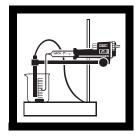
**9.** Continue the titration, recording at least three points on the downward sloping curve and at least three points after the end point has been reached. The latter points will have little change in the LED readings.
