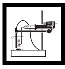
**10.** Continue the titration, recording at least three points on the downward sloping curve and at least three points after the end point has been reached. The latter points will have little change in the LED readings.
