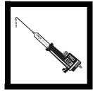
**1.** Insert a clean, straight-stem delivery tube to a Mercuric Nitrate Titration Cartridge. Attach the cartridge to the titrator body. See *General Description, Step-by-Step* for assembly instructions, if necessary. **2.** Flush out the delivery tube by turning the knob until titrant begins flowing from the end of the tube. Wipe the tip and reset the counter to zero.
