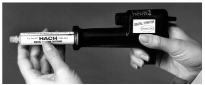
**3.** Remove the polyethylene cap and insert a clean delivery tube into the end of the cartridge until it is tight. See *Figure 3*. Use a straight tube with a hook at the end for hand-held titrations; use a 90° tube with a hook at the end for stationary setups.
