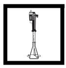
**6.** If the solution turns pink, titrate to a colorless end point. Place the delivery tube tip into the solution and swirl the flask while titrating with sulfuric acid. Record the number of digits required.
