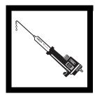
2. Install the Phenylarsine Oxide (PAO), 0.00564 N Cartridge. Flush the Digital Titrator delivery tube by turning the delivery knob to eject a few drops of titrant. Reset the counter to zero and wipe the tip.
