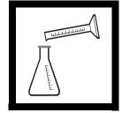
**4.** Use a graduated cylinder or pipet to measure the sample volume from *Table 1*. Transfer the sample into a clean 250-mL Erlenmeyer flask. Dilute to about the 100-mL mark with deionized water, if necessary.
