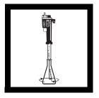
8. Place the delivery tube tip into the solution and swirl the flask while titrating the sample until the color changes from red to the original yellow. Record the number of digits required.
