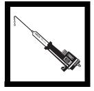
**8.** Turn the delivery knob to eject a few drops of titrant. Reset the counter to zero and wipe the tip.
