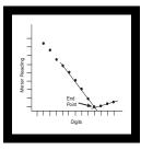
**10.** Using linear graph paper, plot the recorded readings from the Amperometric Titrator on the vertical axis and the corresponding Digital Titrator digits on the horizontal axis. Draw the two best intersecting lines through the points; see *Figure 1*. Determine the number of digits at the intersection of the lines; this is the end point.
