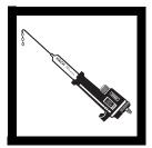
**3.** Turn the delivery knob to eject a few drops of titrant. Reset the counter to zero and wipe the tip.
