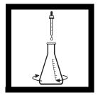
**5.** Add five drops of 5.25 N Sulfuric Acid Standard Solution to the flask. Swirl to mix.
