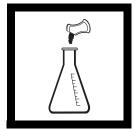
**5.** Add the contents of one Phenolphthalein Indicator Powder Pillow and swirl to mix. The solution should be colorless.
