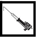
2. Flush the delivery tube by turning the deliver knob to eject a few drops of titrant. Reset the counter to zero and wipe off the tip.
