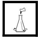
**11.** Add the contents of **12.** Place the delivery one ManVer® 2 Hardness Indicator Powder Pillow (Cat. No. 928-99) or 4 drops of Hardness 2 Test Solution (Cat. No. 425-32). Swirl to mix.
