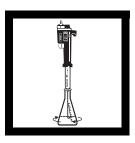
**5.** Add the contents of one ManVer® 2 Hardness Indicator Powder Pillow to the flask and swirl to mix. If color appears. Record the solution turns blue. free chelant is present. Proceed to step 6. If the solution turns red, a deficiency of chelant exists.
