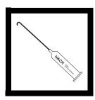
**2.** Insert a clean delivery tube into the titration cartridge. Attach the cartridge to the titrator body. See *General Description*, *Step-by-Step*, for assembly instructions, if necessary.
