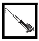
2. Flush the delivery tube by turning the delivery knob to eject a few drops of titrant. Reset the counter to zero and wipe the tip.
