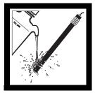
8. Remove the probe arm from the beaker and rinse the platinum wires with deionized water. Adjustment of the electrode response slope is complete.
