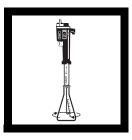
**10.** Place the delivery tube tip into the solution and swirl the flask while titrating with sodium thiosulfate to a pale yellow color.
