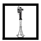
**9.** Continue the titration until the solution changes from dark blue to colorless. Record the number of digits required.
