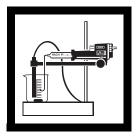
**5.** Place the beaker on the TitraStir<sup>®</sup> Stir Plate and immerse the tips of the probe and delivery tube in the solution. The probe's platinum wires must be submerged. Turn on the stirring motor.
