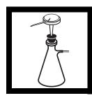
**2.** Using plastic tweezers, position a 0.45 micron membrane filter on top of the funnel stem.
