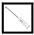
**2.** Insert a clean delivery tube into the appropriate Sodium Hydroxide Titration Cartridge. Attach the cartridge to the titrator body. See *General Description, Step-by-Step*, for assembly instructions.
