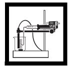
**3.** With minimum agitation, measure 200 mL sample with a clean graduated cylinder and transfer the sample to the beaker. Swirl to mix the reagents with sample.
