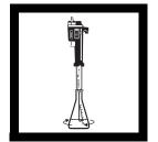
**5.** Place the delivery tube tip into the solution and swirl the flask while immediately titrating with FEAS to a colorless end point. Record the number of digits required.
