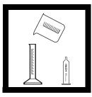
**6.** Select a sample volume and Sodium Thiosulfate Titration Cartridge corresponding to the expected dissolved oxygen (D.O.) concentration from *Table 1*.
