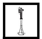
**9.** Place the delivery tube tip into the solution. Swirl the flask while titrating with the sulfuric acid titrant until the solution color changes from purple to orangered. Record the number of digits used.
