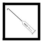
**1.** Select a sample size and a Sodium Hydroxide delivery tube into the (NaOH) Titration Cartridge corresponding to the expected carbon dioxide  $(CO_2)$ concentration; see Table 1.
