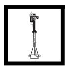
**6.** Place the delivery tube tip into the solution and swirl the flask while titrating with sodium hydroxide until a light pink color forms and persists for 30 seconds. Record the number of digits required.
