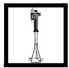
**9.** Continue titrating until the solution turns from blue to colorless. Record the number of digits required.
