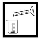
**3.** With minimum agitation, measure 200 mL sample with a clean graduated cylinder. Transfer the sample to a clean 250-mL beaker containing the 50-mm stirring bar supplied with the system.
