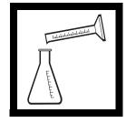
**6.** Accurately measure 20 mL of the prepared sample and transfer it to a 125-mL Erlenmeyer flask.
