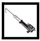
**2.** Turn the delivery knob to eject a few drops of titrant. Reset the counter to zero and wipe the tip.
