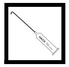
7. Attach a clean straight-stem delivery tube to a 0.2000 N Sodium Thiosulfate Titration Cartridge. Twist the cartridge onto the titrator body. See *General Description*, *Step-by-Step* for assembly instructions, if necessary
