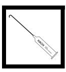
**2.** Insert a clean delivery tube into the appropriate Hydrochloric Acid or Sulfuric Acid Titration Cartridge. Attach the cartridge to the titrator body. See *General Description Section*, *Step-by-Step*, for assembly instructions, if necessary.
