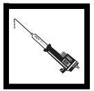
**3.** Flush the delivery tube by turning the delivery knob to eject a few drops of titrant. Reset the counter to zero and wipe the tip.
