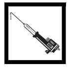
**3.** Flush the delivery tube by turning the delivery knob to eject a few drops of titrant. Reset the counter to zero and wipe the tip.
