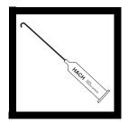
**1.** Insert a clean delivery tube into the Magnesium Chloride Titration Cartridge. Attach the cartridge to the titrator body. See *General Description*, *Step-By-Step*, for assembly instructions.
