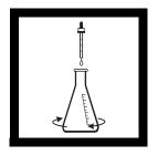
**8.** Add one dropper of Starch Indicator Solution and swirl to mix.
