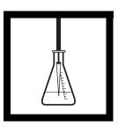
**7.** Use the pipet to dispense 0.2 mL of bleach sample below the solution level in the flask.
