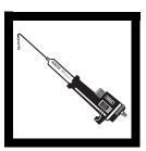
2. Hold the Digital Titrator with the cartridge tip pointing up. Turn the delivery knob until a few drops of titrant are expelled. Reset the counter to zero and wipe the tip.
