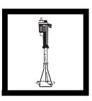
**6.** Place the delivery tube tip into the solution and swirl the flask while titrating with sodium hydroxide from yellow to blue-violet (pH 3.7). Record the number of digits required.
