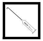
**1.** Insert a clean delivery tube into the 8.00 N Sulfuric Acid Titration Cartridge. Attach the cartridge to the titrator body.
