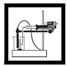
1. Set-up the Amperometric Digital Titrator System as in *Phase 1: Adjusting the Electrode Response Slope* if it has not already been done. Reset the Digital Titrator counter to zero and wipe the tip.
