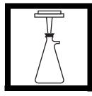
**1.** Attach the filter funnel stem to a 1000-mL filtering flask.
