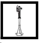
7. Place the delivery tube tip into the solution and swirl the flask while titrating with the iodateiodide to a permanent blue end point. Record the number of digits required. Digits Digit Required Multiplier = mg/L Sulfite (SO₃<sup>°</sup>)
