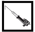
**3.** Turn the delivery<br/>knob to eject a few drops<br/>of titrant. Reset the<br/>counter to zero and wipe<br/>the tip.**4.** Use a graduated<br/>cylinder or pipet to<br/>measure the sample<br/>volume from *Table*<br/>Transfer the sample
