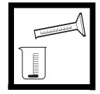
**3.** Using a graduated cylinder, measure 200 mL of deionized water into a clean 250-mL beaker. Place the 50-mm stirring bar supplied with the system
