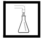
**4.** Collect a water sample directly into the titration flask by filling to the appropriate mark.
