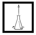
**8.** Add one dropper of starch indicator solution and swirl to mix. A dark blue color will develop.
