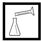
**3.** Use a graduated cylinder to measure the 50 mL of clear sample into a 125-mL Erlenmeyer flask.
