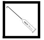
**1.** Insert a clean delivery tube into the 2.26 N Thiosulfate Titrant Solution cartridge. Attach the cartridge to the titrator body.
