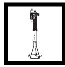
**7.** Place the delivery tube tip into the solution and swirl the flask while titrating with sodium thiosulfate until the solution is a pale yellow.
