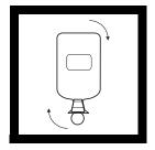
**4.** Wait until the floc in the solution has settled and the top half of the solution is clear. Again invert the bottle several times and wait until the floc has settled.
