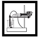
**8.** Using the Digital Titrator delivery knob, dispense the PAO titrant Solution in 5-10 digit increments while noting the downward reading.
