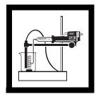
**5.** Place the beaker on the TitraStir Stir Plate and immerse the tips of the probe and delivery tube in the solution. The probe's platinum wires must be submerged. Turn on the stirring motor.
