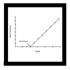
**9.** Using linear graph paper, plot the recorded readings from the Amperometric Titrator on the vertical axis and the corresponding Digital Titrator digits on the horizontal axis. Draw the two best intersecting lines through the points plotted. See Figure 1. Determine the number of digits at the intersection of the lines. This is the *standard* end point.
