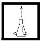
**11.** Add two 1-mL droppers of Starch Indicator Solution and swirl to mix.
