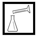
**4.** Use a pipet or graduated cylinder to measure the sample volume from *Table 2*. Transfer the sample into a 125-mL Erlenmeyer flask and dilute to about the 50-mL mark with deionized water.
