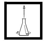
**4.** Using the 1-mL calibrated dropper, add 2 mL of Hardness 1 Buffer Solution to the flask and swirl to mix.
