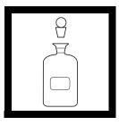
**3.** Immediately insert the stopper so air is not trapped in the bottle. Invert several times to mix.
