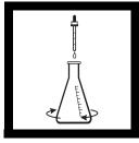
**9.** Place the delivery tube tip into the solution titrating with the thiosulfate titrant until the solution is pale yellow.
