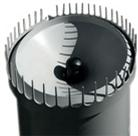
**Bird Guard:** The bird guard prevents wild or feral birds from perching or roosting and thus increases accuracy by stopping bird feces from dropping inside the gauge funnel.
