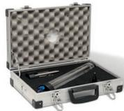
**Portable Field Calibration Device (FCD):** The FCD effectively enables field technicians to run functional tests and calibrations of any given rain gauge in the field avoiding dismantling of TBRG's, reducing TBRG downtime and thereby saving time and money.
