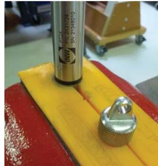
*Cableless Sensor - gripping on knurled area*
