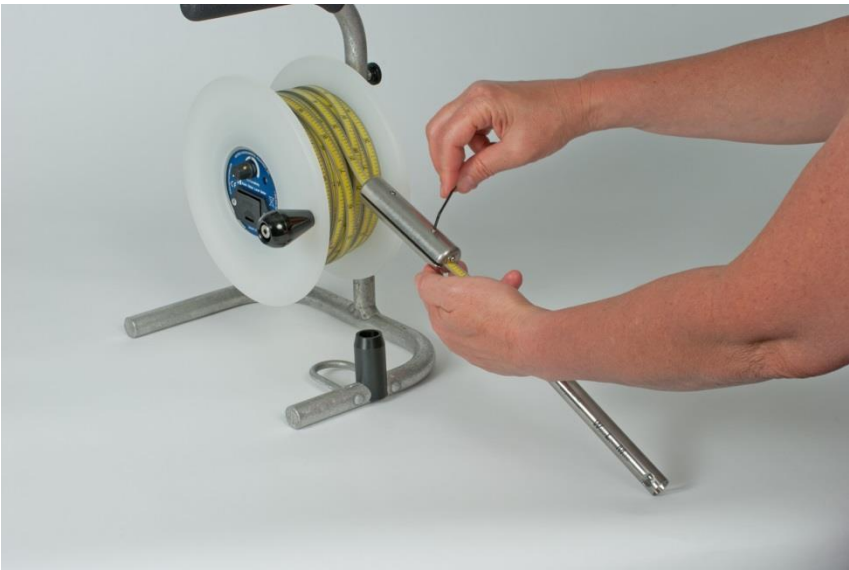
Figure 2-3 Tightening (Optional) Tape Weight
