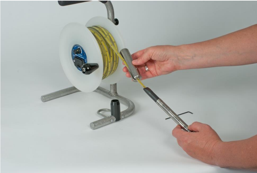
Figure 2-2 Fitting (Optional) Tape Weight
