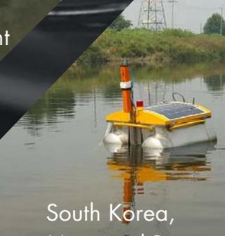
Optical non-contact and autonomous sensor for real-time detection of oil contamination - UV fluorescence technology
