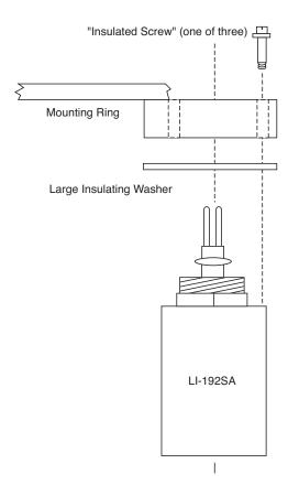
Figure 1-5. Use an insulating washer in heavily ionic water.
