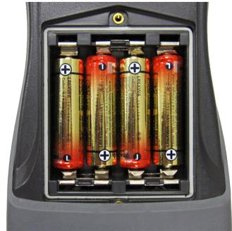
Figure 1-1. "AA" batteries installed.
