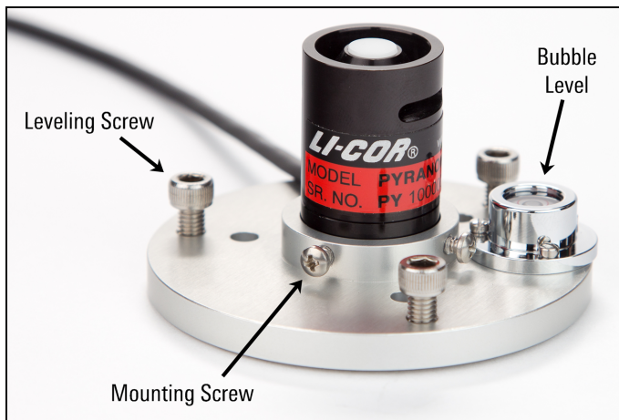
Figure 2-1. LI-200R Pyranometer mounted in the 2003S Mounting and Leveling Fixture.
