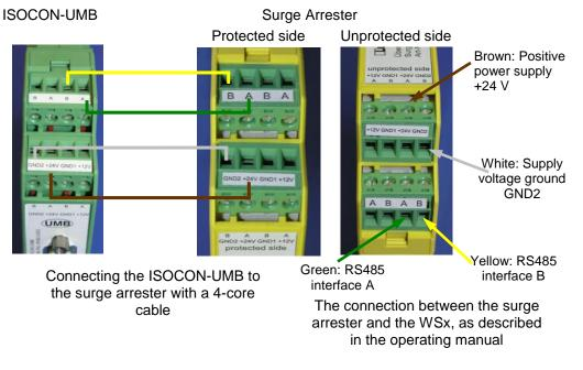
Either an additional surge arrester must be provided on the WSx heating power supply **or** both heating and sensor power supply must be powered in parallel using the same surge arrester.
