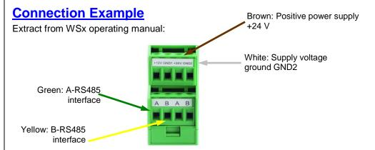
The wiring required to connect the WSx to the surge arrester is as follows:
