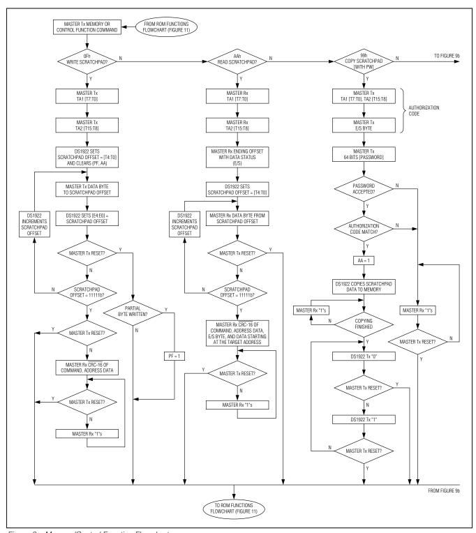
Figure 9a. Memory/Control Function Flowchart
