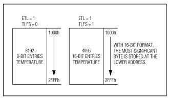
Figure 7. Temperature Logging
