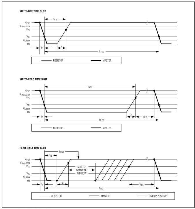
Figure 13. Read/Write Timing Diagrams
