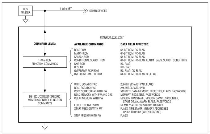
Figure 2. Hierarchical Structure for 1-Wire Protocol
