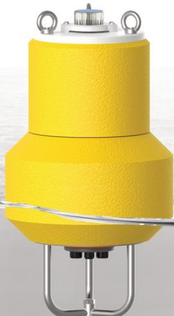
The NexSens **CB-50** Data Buoy is designed for quick deployment in emergency response situations including industrial spills and natural disasters. The buoy can be deployed from small boats, large vessels or even helicopters, making it the ideal choice for applications where water needs to be monitored at a moment's notice. Compatible instruments include turbidity sensors, dissolved oxygen sensors, hydrocarbon sensors, fluorometers, multi-parameter sondes, pressure transducers, and more.
