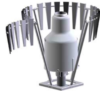
Movable segment for safe access to precipitation gauge
