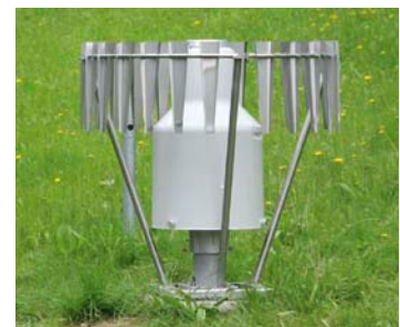
Movable segment for safe access to precipitation gauge
