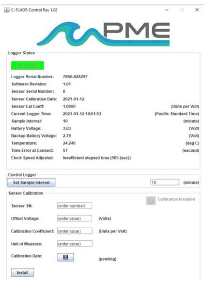
The current Logger sample interval will be displayed next to the Set Sample Interval button. If this interval is acceptable the interval need not be set.
