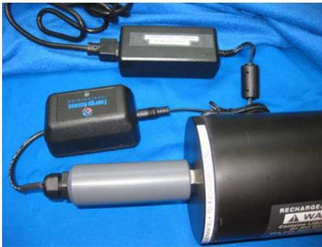
Connect the battery charger. The charger will require power from a power supply. The charger has a LED light indicating the status of the charging.
