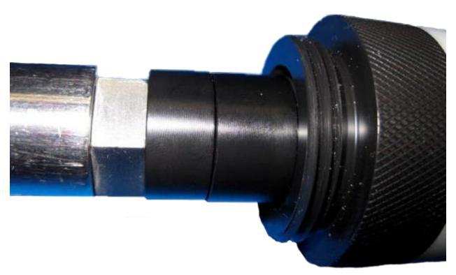
Slide the sensor support (middle-right in first picture) over the sensor. Note this part has an internal o-ring that comes against the sensor. This is not a water-proof seal. Its purpose is to firmly secure the sensor within the support. Next screw the sensor guard (middle left in first picture) onto the sensor support. The completed assembly is shown in the picture below.
