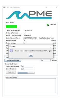
A "Please place sensor in calibration standard of <Calibration Value> (<Unit of Measure>)" dialog appears. In the screen shot above the value of 400 (ppb) is displayed. This information is taken from the Unit of Measure and Calibration Value text boxes and will be whatever is entered in the boxes.
