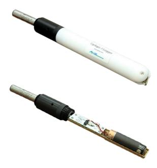
The logger circuitry is contained in a waterproof housing that must be opened. The housing is opened by unscrewing the white pressure housing from the black end cap. Turn the pressure housing counter clockwise relative to black end cap. Close by reversing this procedure after being sure that the o-ring is free from debris. Lube o-ring occasionally with grease intended for buna-n o-ring material.
