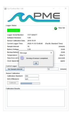
When this is completed a Zeroing of sensor completed dialog appears. Click OK.
