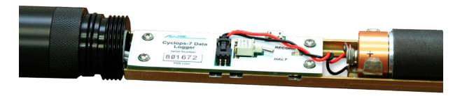
The **LED Light** is a LED that can display either red or green light. This is used to indicate different features described in Chapter 1 in this manual.
