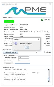
When this is completed a "Calibration completed" dialog window appears along with the actual calibration results.
