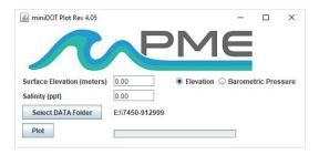
The miniDOT Plot program plots the files recorded by the miniDOT Clear Logger. The program reads all the miniDOT Clear Logger files in a folder, except the CAT.txt file. The program will also compute air saturation from the dissolved oxygen measurements. To do this, the program must know the air pressure and salinity. It calculates air pressure based on elevation of the water surface above sea level or uses the
