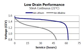
The figure to the left gives a general idea of terminal voltage vs. lifetime. Service life in hours is incorrect since miniDOT Clear Logger draws far less than 50 mA continuously, but the general shape of the voltage vs. time gives an estimate of life remaining. This plot is taken from the manufacturer's specification. The plot is for a single battery. The miniDOT Clear Logger halts operation at a total of 2.4 Volts.
