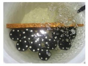
Record measurements for several hours or a day, but in any event long enough for the miniDOT Clear Logger's temperature to come to equilibrium with the water. During the experiment, find the local air pressure, either from measurements or from a local weather station. Watch out... weather stations often report barometric pressure referenced to sea level. You must determine the absolute barometric pressure at your elevation.
