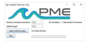
The miniDOTPlot program plots the files recorded by the miniDOT Logger. The program reads all the miniDOT Logger files in a folder, except the CAT.txt file. The program will also compute air saturation from the dissolved oxygen measurements. To do this, the program must know the air pressure and salinity. It calculates air pressure based on elevation of the water surface above sea level or uses the barometric
