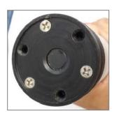
Position the Copper Plate faced down so that the notches in the Copper Plate perfectly align over sensing foil and over the screw holes.
